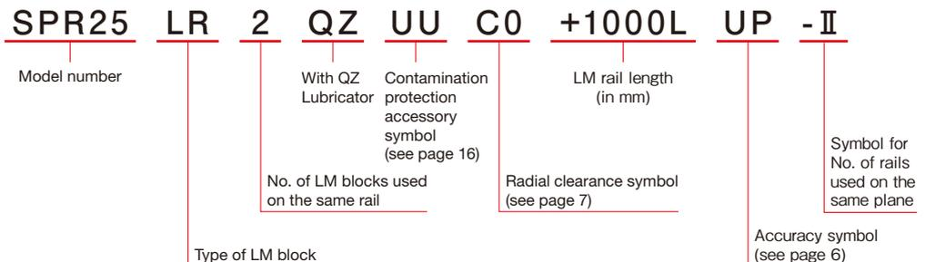
Note) This model number consists of a set of LM blocks and LM rails. (At least two sets are required when using two rails in parallel.)
